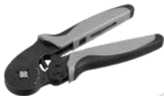
92145 For cord-end terminals SQUARE crimp Single wire 0,08 - 10,0 mm 2 Twin wire 2x0,25 - 2x4,0 mm 2
