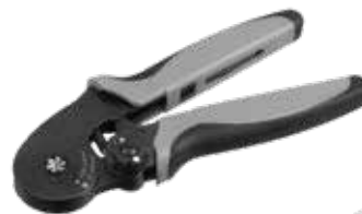
92146 For cord-end terminals HEXAGONAL crimp Single wire 0,08 - 16,0 mm 2 Twin wire 2x0,25 - 2x6,0 mm 2
