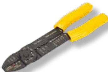
KH-507 Multi-tool for insulated and non-insulated (brazed seam only) terminals 0,5~6,0 mm 2 Stripping 0,75~6,0 mm 2
