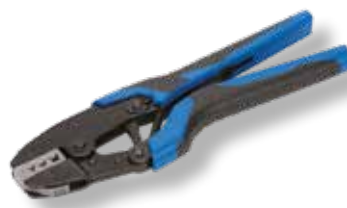
MH-2P Crimping tool for cord end terminals 6,0-16,0 mm 2
