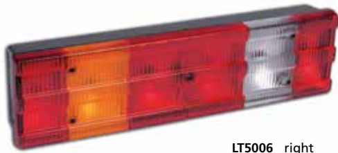
LT5006 right bulbs 4xP21W, 2xR10W LT5007 left bulbs 4xP21W, 3xR10W
