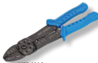
MEB-900C Multi-tool for non-insulated (brazed seam only) and open barrel terminals 0,5~6,0 mm 2 Stripping 0,75~6,0 mm 2
